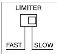
The integrated limiter provides reliable protection against signal clipping and has a switchable time constant. Leaving the switch set to SLOW is recommended for general use (factory pre-set status).
